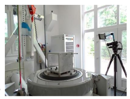
Figure 2 - The picture of the Vibration **Test System**
