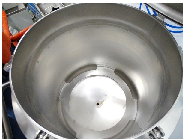
Figure 13. Inside view of the overpressure vessel with the bottom tray for the DUT
