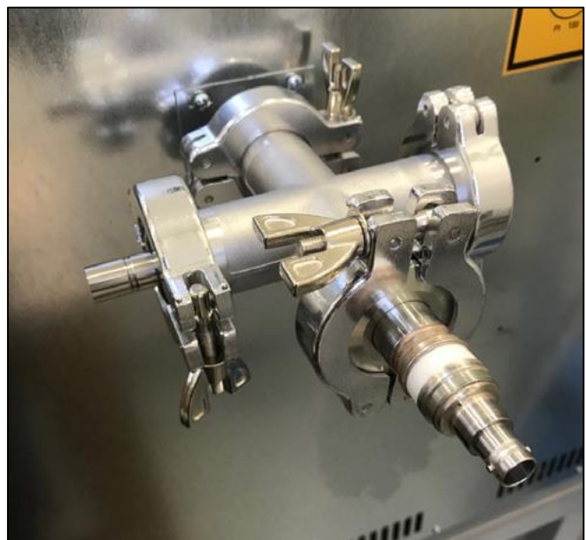
Figure 8 – The picture of the Vacuum Bakeout Chamber electrical interfaces (outside)
