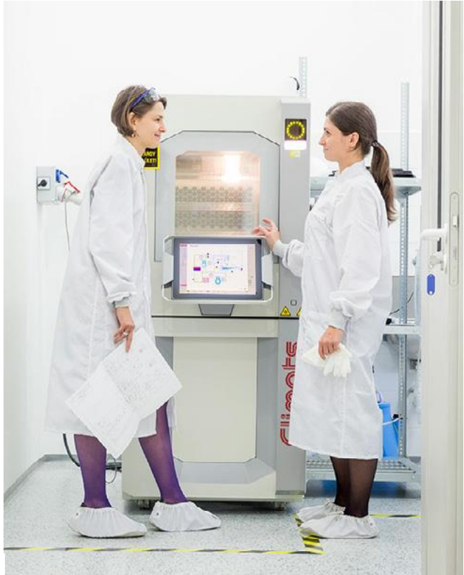
Figure 6 – The picture of the Climate Test Chamber
